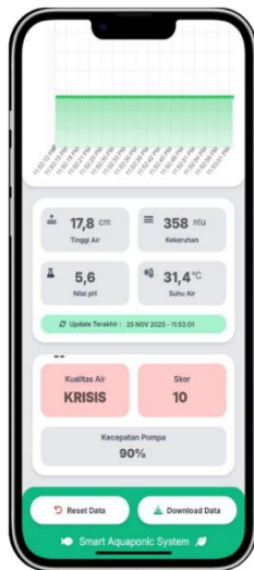
Gambar 11. Tampilan Dashboard Monitoring Suhu, pH, Kekeruhan, dan Level Air
