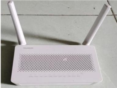
**Gambar 3. Router Huawei HG8145V5**
