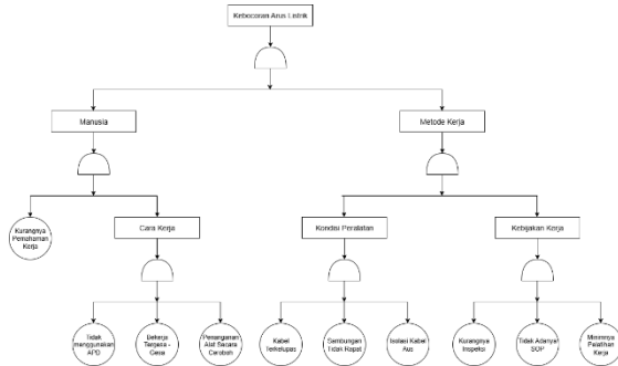
Gambar 3. Fault Tree Analysis Kebocoran Arus Listrik
