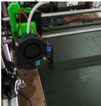
Gambar 10 Proses Touching Leveling
